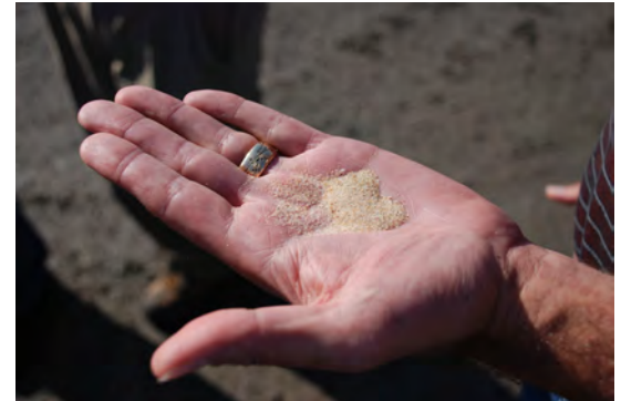
Fine-grained silica sand is mixed with chemicals and water before being pumped into rock formations to prevent the newly created artificial fractures from closing after hydraulic fracturing is completed. Photo: Bill Cunningham, U.S. Geological Survey
